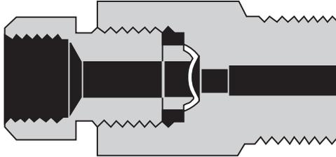
The male inlet design can be inserted directly into the tubing connections of valves and various fittings such as tees and crosses, or located in pressure vessels.
